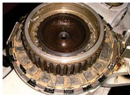
C-5 landing gear is challenged by corrosion, which can be minimized by proper grease selection.
